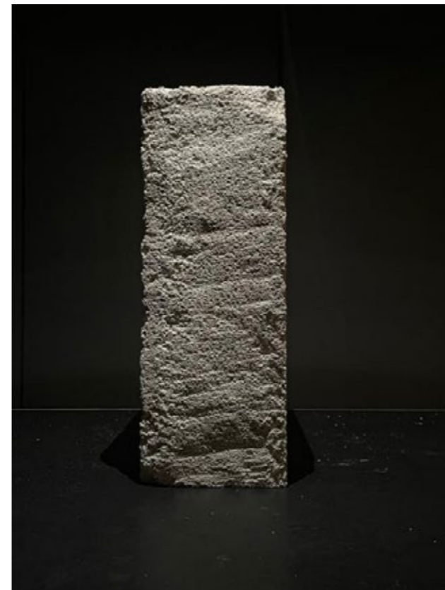
fig 21. waterjet cut surface marks
