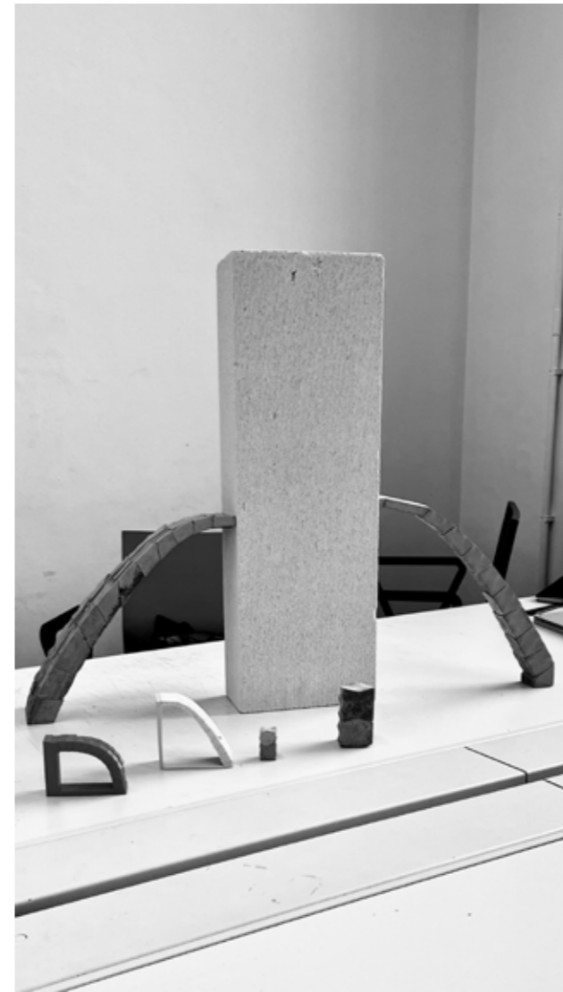
fig 18. final arch, previous pattern test, casting tests and 3D print tests
