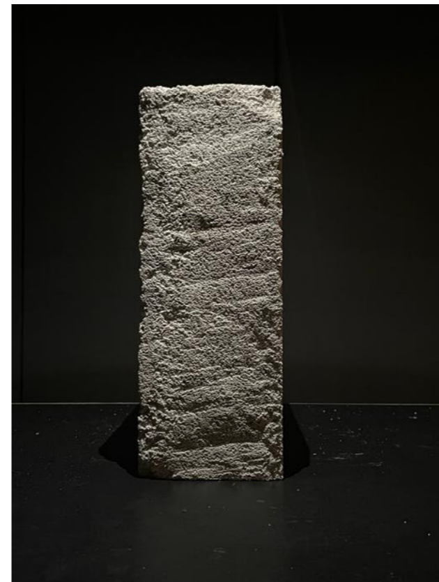
fig 21. waterjet cut surface marks
