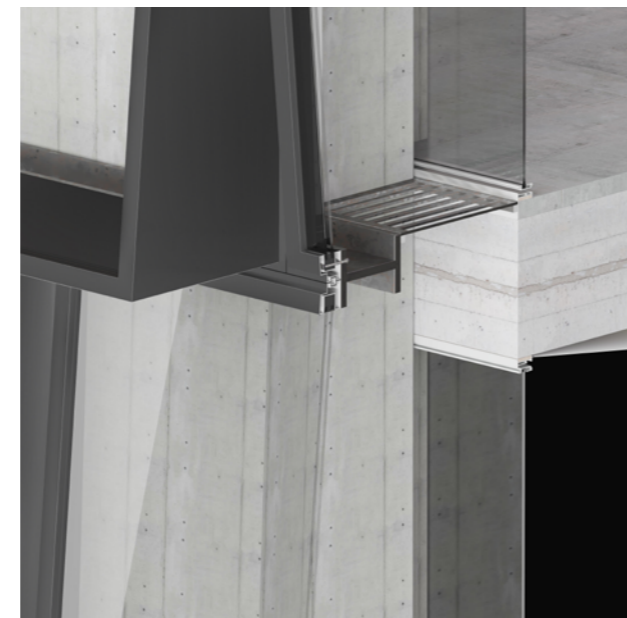
fig 3. 3D facade connection detail
