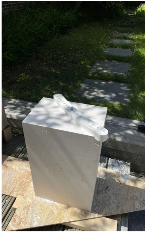
block with 3D printed drill guide
