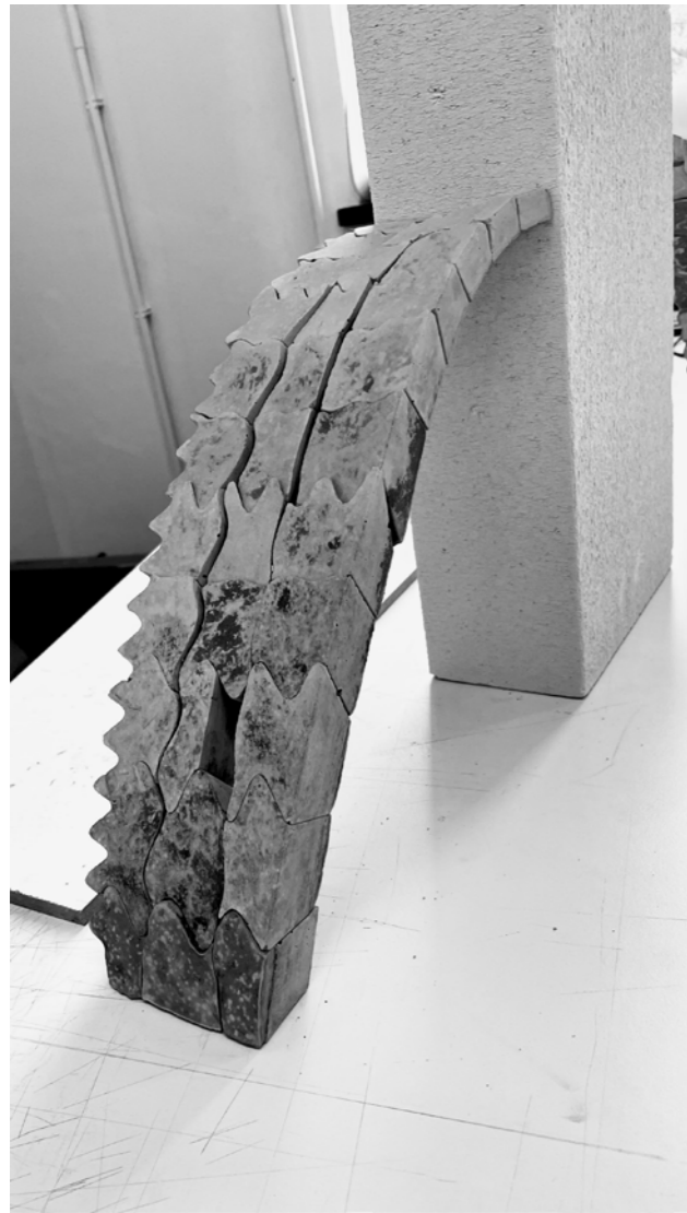
fig 16, 17. cast concrete model to test the connection pattern
